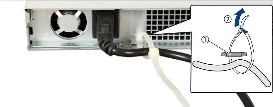
Figure 4: Using cable ties
