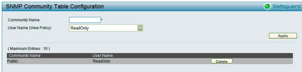
Figure 56 – System > SNMP Settings > SNMP Community Table
