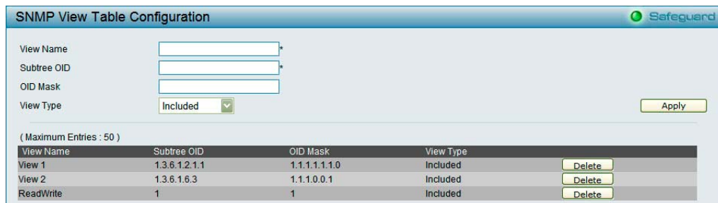
Figure 55 – System > SNMP Settings > SNMP View Table
