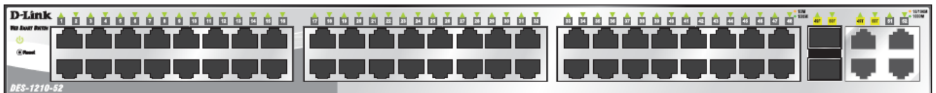
Figure 7 – DES-1210-52 Front Panel
