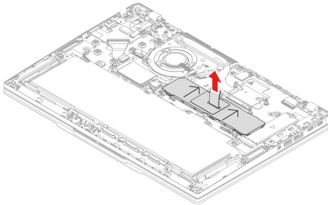
Step 2. Install the memory module shielding cap as shown below.
