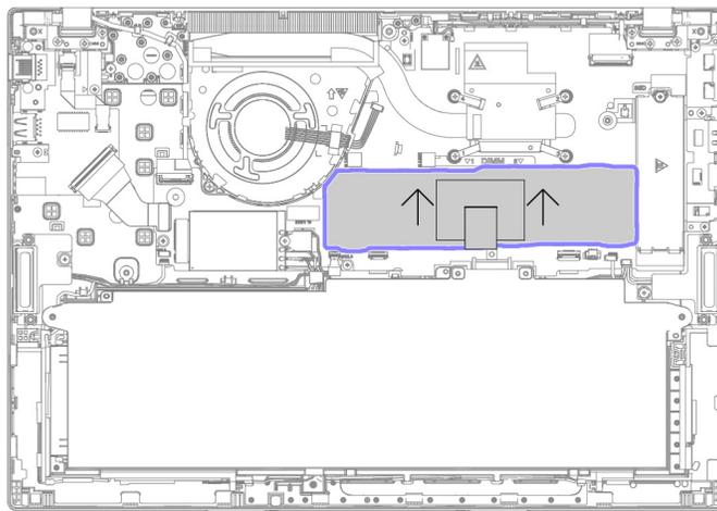
Step 1. Remove the memory module shielding cap as shown below.
