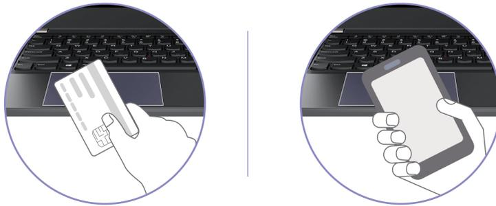
**Note:** Ensure that the NFC card is in NFC Data Exchange Format (NDEF), otherwise the card cannot be detected.
