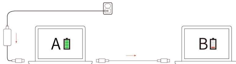
**Note:** The actual charging speed of your computer depends on many factors, such as the remaining battery power of the computers, the wattage of the ac power adapter, and whether you are using the computers.
