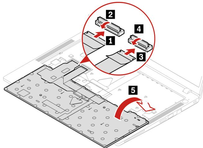
Step 2. Insert the keyboard into the keyboard bezel as shown. Ensure that the top edge of the keyboard (the edge that is close to the display) is under the keyboard bezel.
