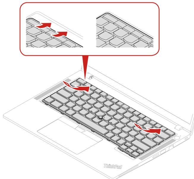
Step 3. Slide the keyboard in the direction as shown. Ensure that the latches are secured under the keyboard frame.
