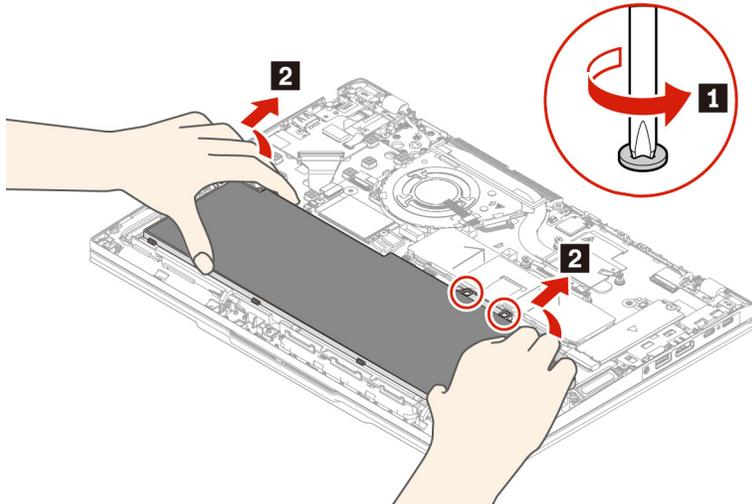
Step 2. Before installing the built-in battery, thoroughly check the battery compartment and ensure that there are no foreign or sharp objects that could cause damage to the battery.
