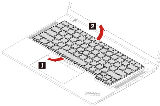
Step 4. Put the keyboard on the palm rest as shown and detach the connectors. Then, remove the keyboard.
