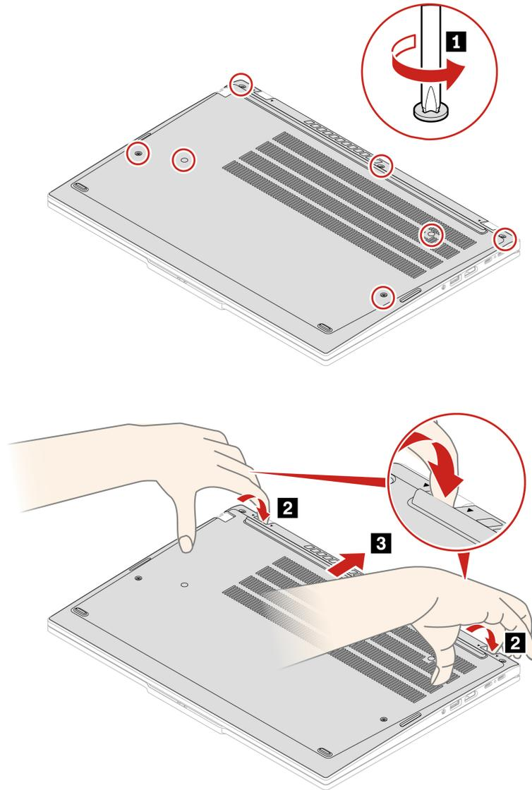
Step 2. Install the base cover assembly as shown below.
