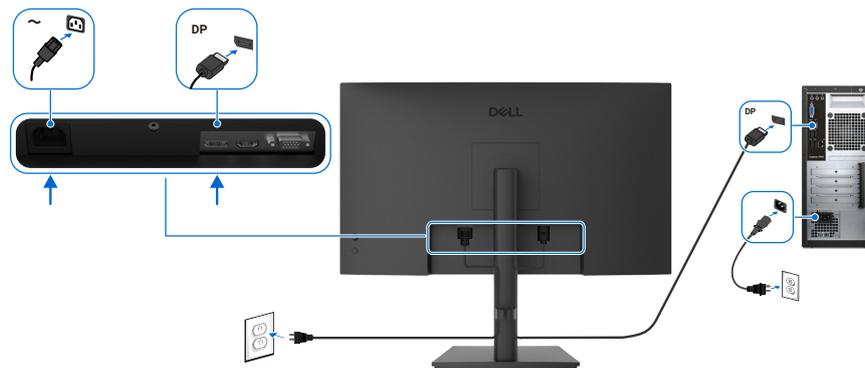
**Figure 23.** Connecting DisplayPort cable
