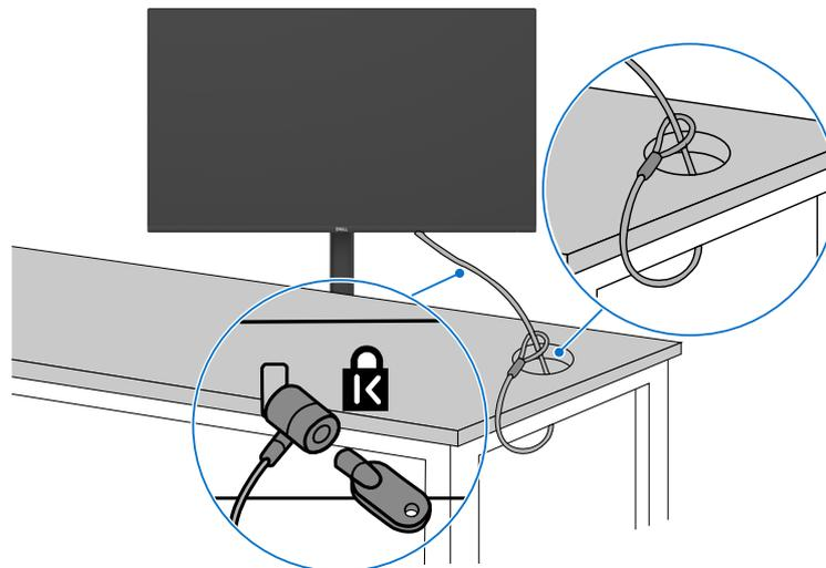
Figure 27. Securing your monitor using Kensington lock
