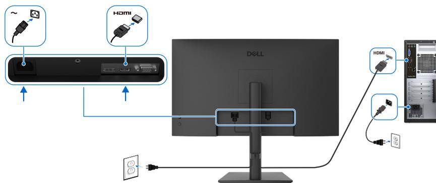
**Figure 24.** Connecting HDMI cable
