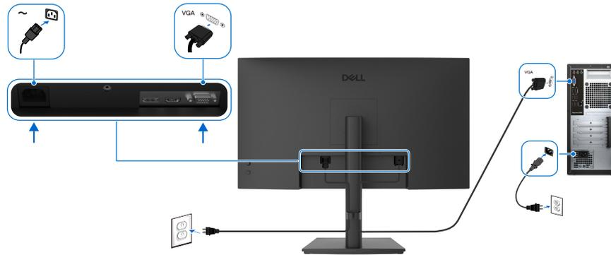
Figure 25. Connecting the VGA cable
