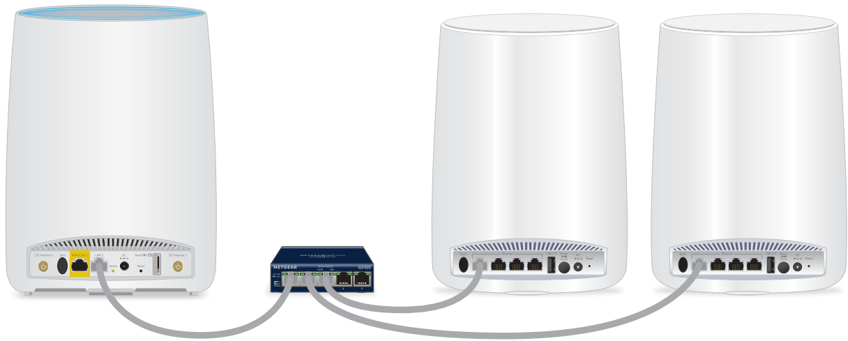
Figure 4. Ethernet backhaul connection using a switch
